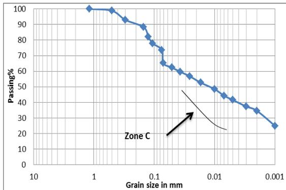
Fig. 6: Granular size analysis for the station (4).
