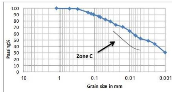
Fig. 3: Granular size analysis for the station (1).
