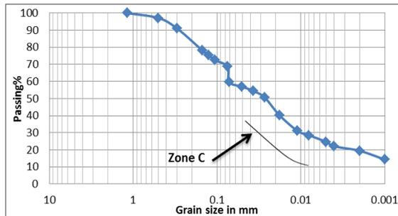
Fig. 4: Granular size analysis for the station (2).
