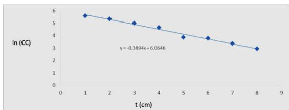
**Fig. 5: Relation between Ln (CC) and thickness for Fe sheets**
