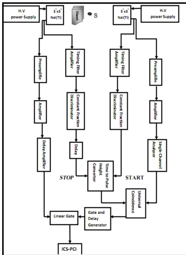
Fig. 2: Block diagram of the gamma-gamma coincidence spectrometer
