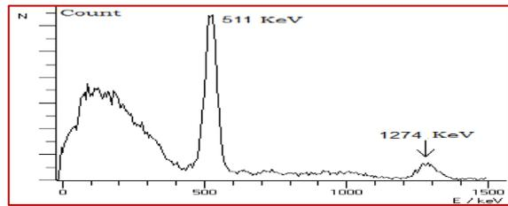
Fig 1: Typical gamma spectrum for Na-22 source obtained with NaI (TI) detector [7].
