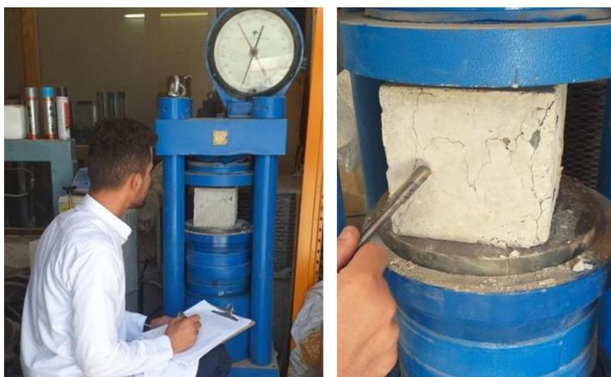
**Plat 5: The process of checking the compressive strength of concrete cubes**
