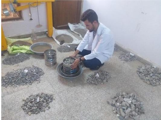
**Plat 2: grain size analysis test process for coarse and fine aggregates**
