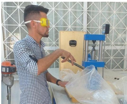
**Plat 4: Point Load Test for samples of the study area**
