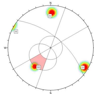
Fig. 9: Planar sliding in station 1
