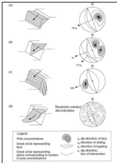
**Fig. 3: The main types of Failures [8] where (a) planar sliding, (b) wedge sliding(c) Toppling(d) rotational sliding**
