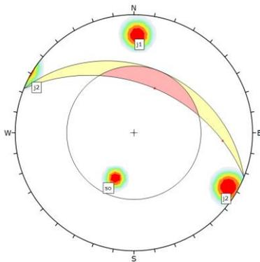
Fig. 11: wedge sliding in station 1
