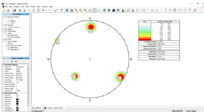
Fig. 5: the projection of the slope face and discontinuities
