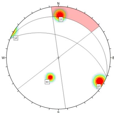
Fig. 13: flexural toppling sliding in station 1
