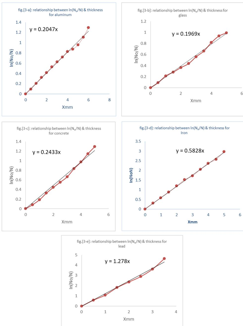
**Fig. 3: The relationship between  $\ln(N_0/N)$  and thickness for materials**
