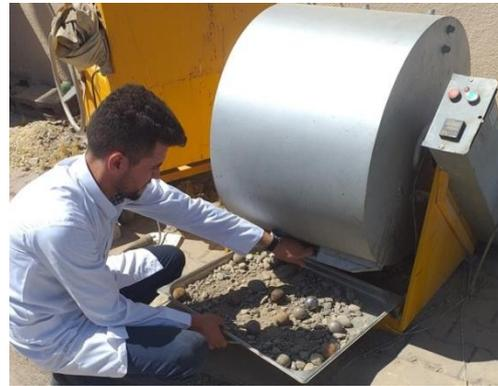
**Plate 3: showing the Los Angeles test process**
