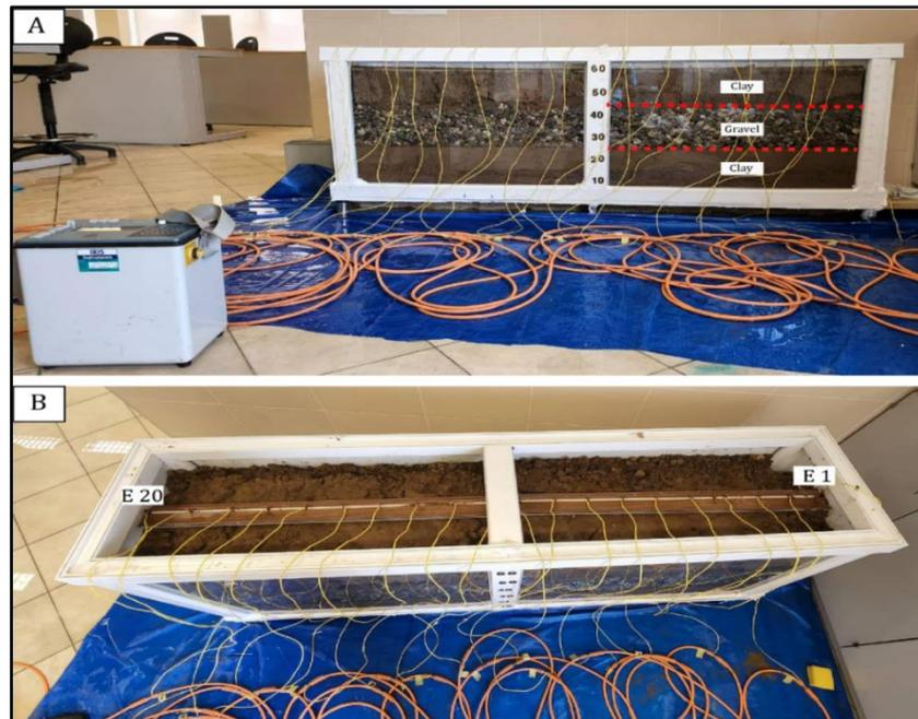
Fig. 4 A: Side view of the laboratory geological model. B: Top view of the model.
