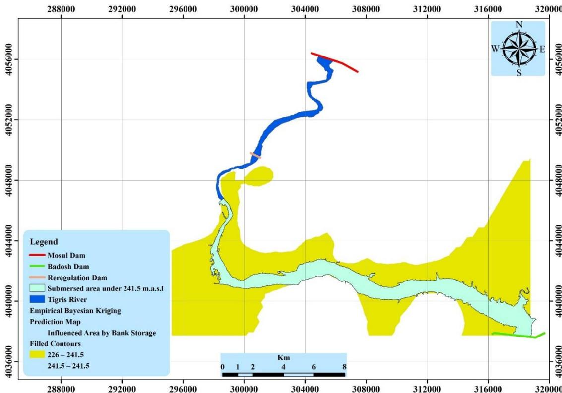
Figure 7: Scenario of the effect of bank storage when the water level in the reservoir is (241.5) m (a.s.l)
