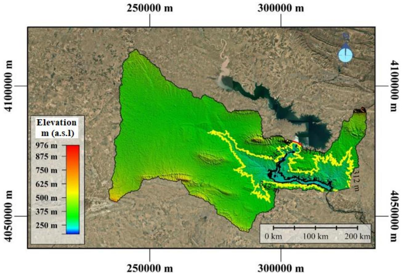
**Figure 2:** Digital elevation model of the river within the reservoir boundaries, marked by the maximum operational level of the reservoir (in black) and the maximum flood level when the breakdown of Mosul Dam happens (in yellow)
