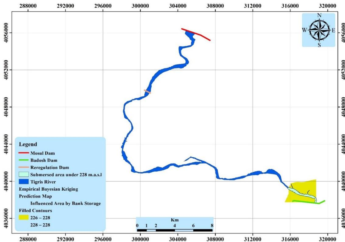
**Figure 5:** Scenario of the effect of bank storage when water level in the reservoir is (228) m (a.s.l)
