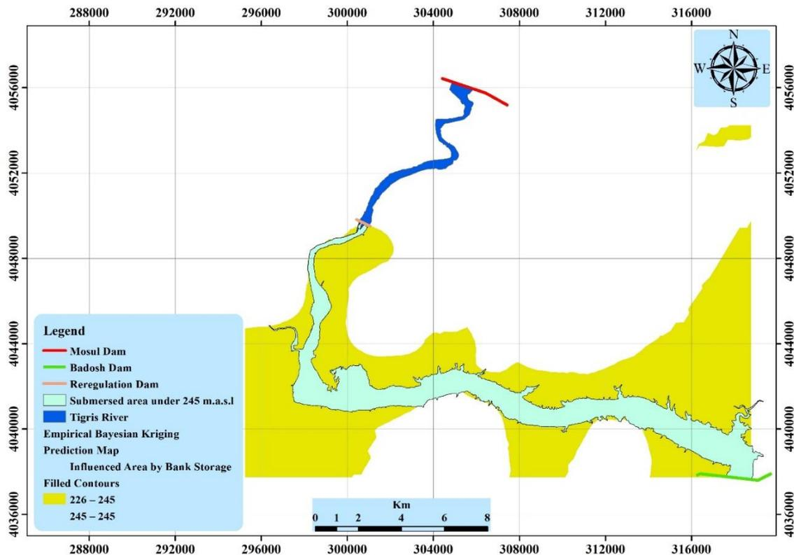
Figure 8: Scenario of the effect of bank storage when the water level in the reservoir is (245) m (a.s.l)
