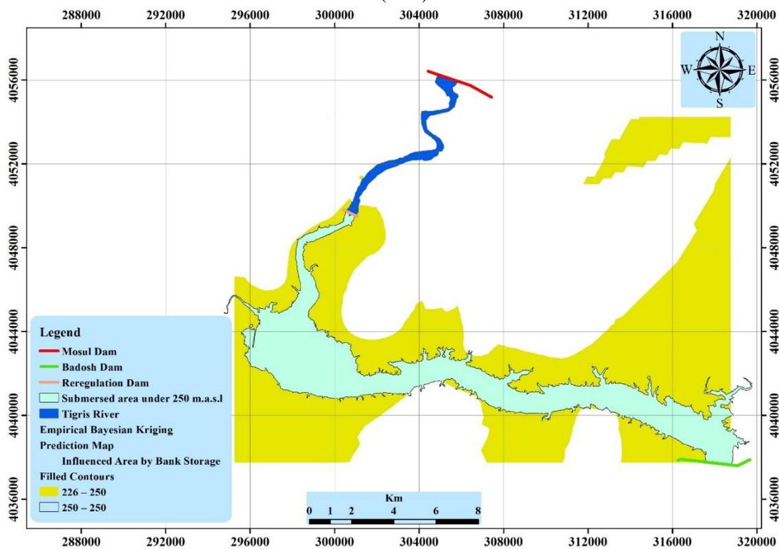
Figure 9: Scenario of the effect of bank storage when the level in the reservoir is (250) m (a.s.l)
