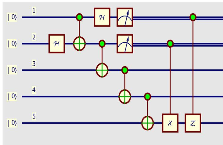
**Figure (4):** the entanglement state for four-basis states of five qubits after applying Bell state measurement.
