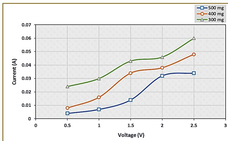
Fig. 5: Influence of NaCl concentration on the I-V curve.
