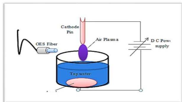
**Fig. 1: Experimental setup of Pin-Liquid configuration**
