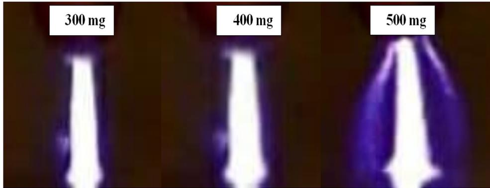
Fig. 3: Typical images of the influence of NaCl concentration on the discharge channel in the gap between (pin-liquid surface).
