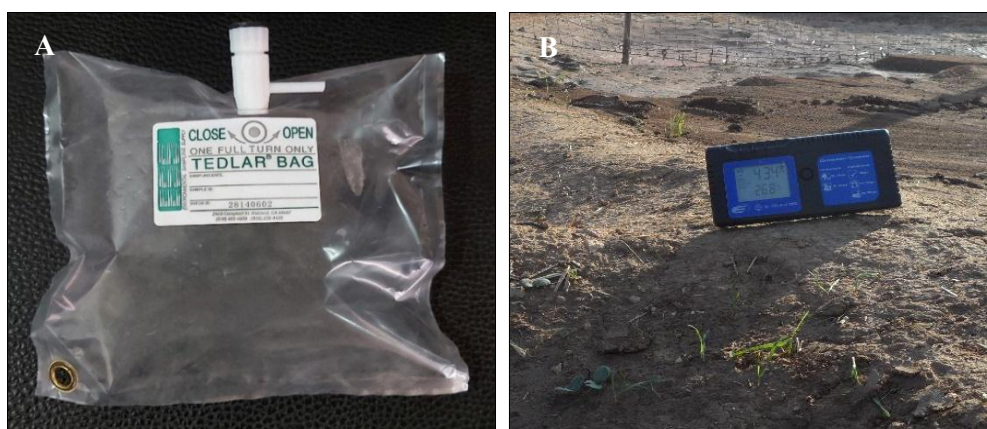
Fig. 6: A) Tedlar Bags ESS for gas composition analysis B) \text{CO}_2 meter Air \text{CO}_2\text{ntrol} 3000
