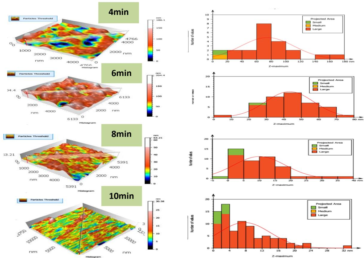
Fig.4 PbO's structural characteristics at different bombardment times (4, 6, 8, and 10 min)
