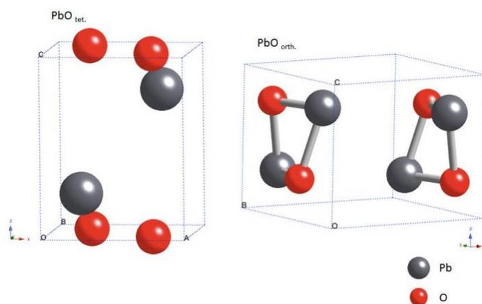
**Fig. 1** A diagram displaying the PbO crystal structure [15]
