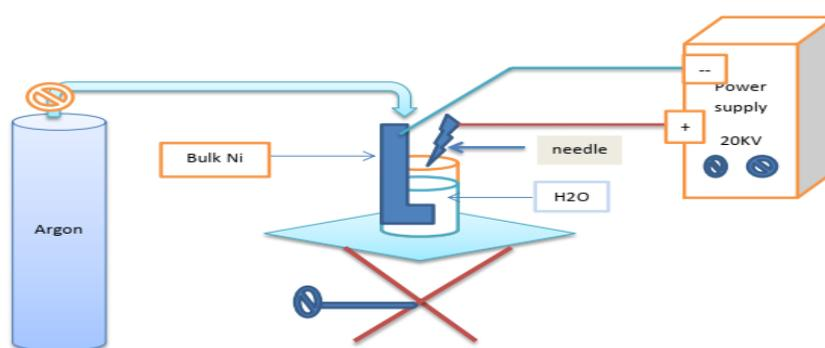
*Fig.2 Explain the operation of the induced plasma -jet*
