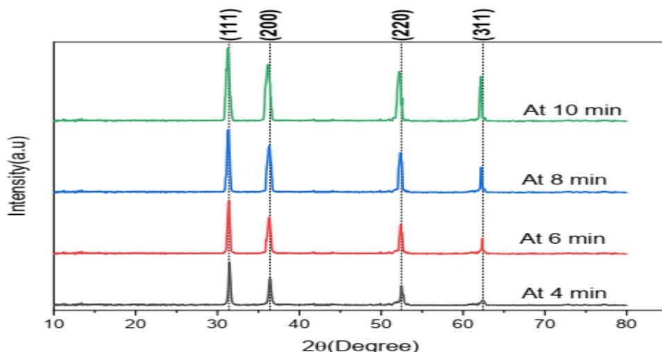
Fig.5 displays the induced plasma bombardment-induced X-ray diffraction of PbO metal oxide after various times of preparation.
