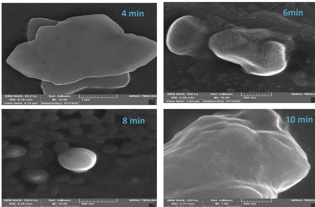
Fig.6 SEM images of PbO prepared at different bombardment periods (4,6,8,10 min)
