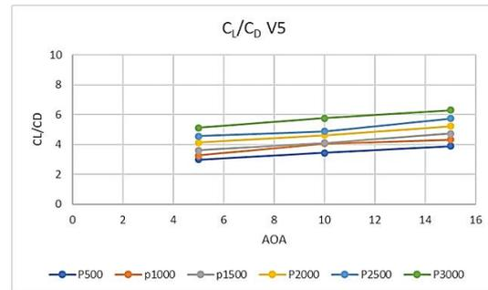
**Fig. 8: Lift-to-Drag Ratio ( $C_L/C_D$ ) for Different Grit Sizes at 5 m/s.**
