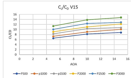
**Fig. 6: Lift-to-Drag Ratio ( $C_L/C_D$ ) for Different Grit Sizes at 15 m/s.**
