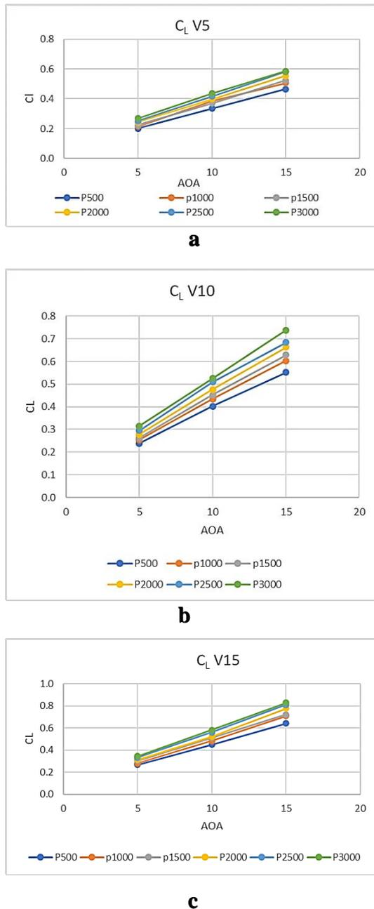
**Fig. 4: Lift Coefficient ( $C_L$ ) for Different Grit Sizes at Various Angles of Attack and Flow Speed: (a) 5 m/s, (b) 10 m/s, (c) 15 m/s.**
