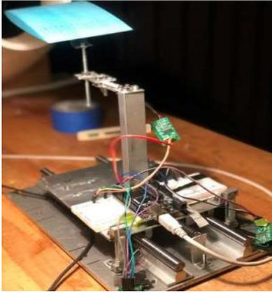
**Fig. 3: Force balance setup for measuring lift and drag forces.**
