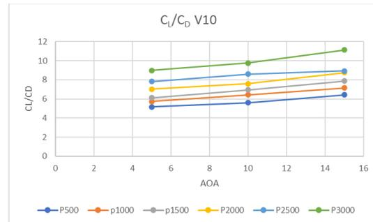
**Fig. 7: Lift-to-Drag Ratio ( $C_L/C_D$ ) for Different Grit Sizes at 10 m/s.**
