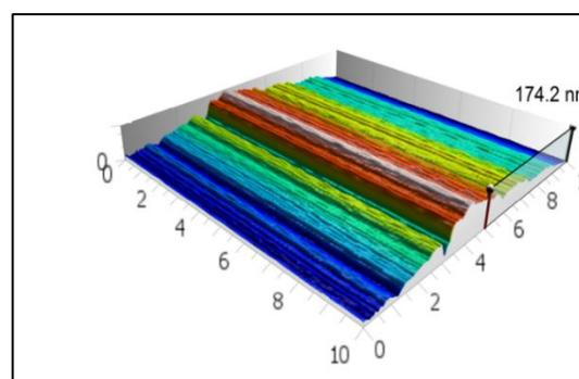
**Fig. 7:** Cross-section image of PS prepared by ECE technique with a constant time of 25 min. And constant current density 25 mA /cm<sup>2</sup> with HF: ethanol mixing B: (1:6)
