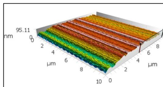
**Fig. 6:** Cross-section image of PS prepared by ECE technique with a constant time of 25 min. And constant density of current 25 mA /cm<sup>2</sup> with HF: ethanol mixing A: (1:9)
