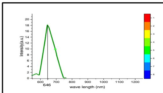
**Fig. 12: PL image of PS wafer prepared by ECE technique with a constant time of 25 min. And constant density of current 25 mA /cm<sup>2</sup> with HF: ethanol mixing A: (1:9)**
