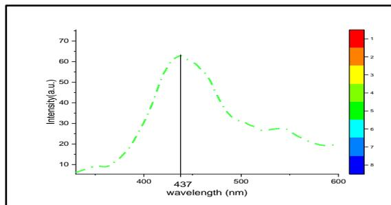
**Fig. 14:** PL image of PS wafer prepared by ECE technique with a constant time of 25 min. And constant density of current  $25 \text{ mA/cm}^2$  with HF: ethanol mixing C: (1:3)
