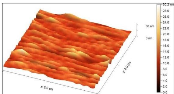
Fig. 2: AFM image of PS prepared by ECE technique with a constant time of 25 min. and constant density of current 25 mA /cm<sup>2</sup> with HF: ethanol mixing A: (1:9)
