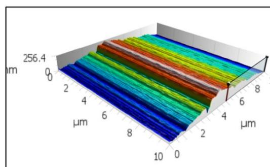
**Fig. 8:** Cross-section image of PS prepared by ECE technique with a constant time of 25 min. And constant current density 25 mA /cm<sup>2</sup> with HF: ethanol mixing C: (1:3)
