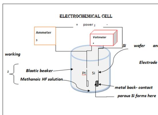
Fig. 1: The porous silicon fabrication system (electrochemical cell) [10]
