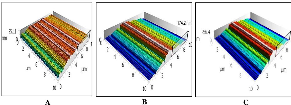
**Fig. 9: Cross-section image of PS prepared by ECE technique with a constant etching time of 25 min. and constant density of current 25 mA /cm<sup>2</sup> with HF: ethanol mixing (A-1:9, B-1:6, C-1:3)**
