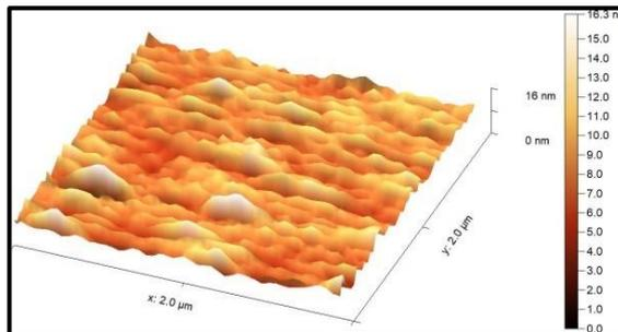
Fig. 3: AFM image of PS prepared by ECE technique with a constant time of 25 min. and constant density of current 25 mA /cm<sup>2</sup> with HF: ethanol mixing B: (1:6)
