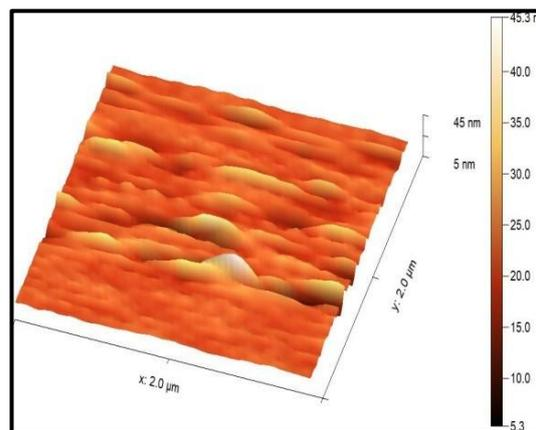
Fig. 4: AFM image of PS prepared by ECE technique with a constant etching time of 25 min. and constant density of current 25 mA /cm<sup>2</sup> with HF: ethanol mixing C: (1:3)
