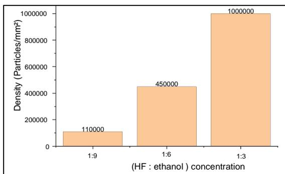
**Fig. 10: The mixing aggregation on the density of particles formed on the surface**
