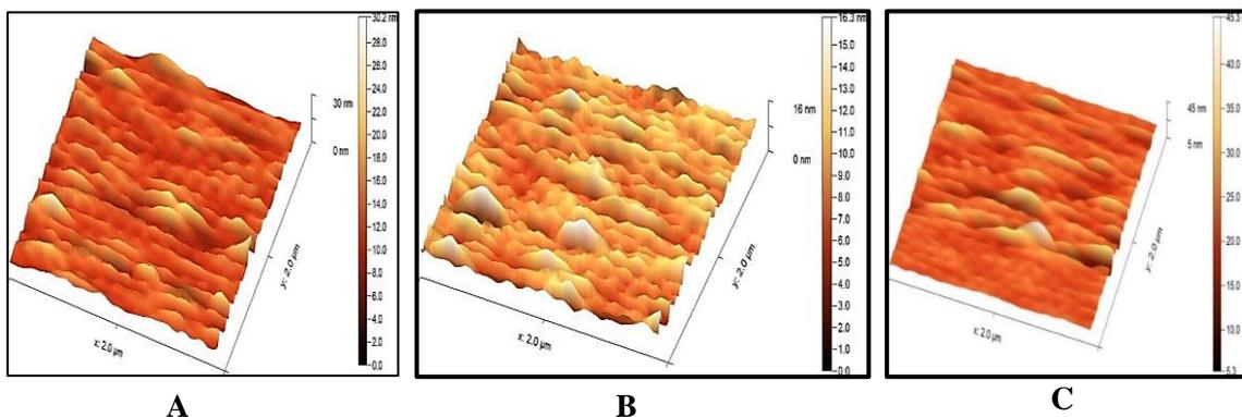
Fig. 5: AFM images of PS prepared by ECE technique with a constant etching time of 25 min. and constant density of current 25 mA /cm<sup>2</sup> with HF: ethanol mixing (A-1:9, B-1:6, C-1:3)
