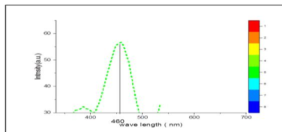
**Fig. 13: PL image of PS wafer prepared by ECE technique with a constant time of 25 min. And constant current density 25 mA /cm<sup>2</sup> with HF: ethanol mixing B:(1:6)**
