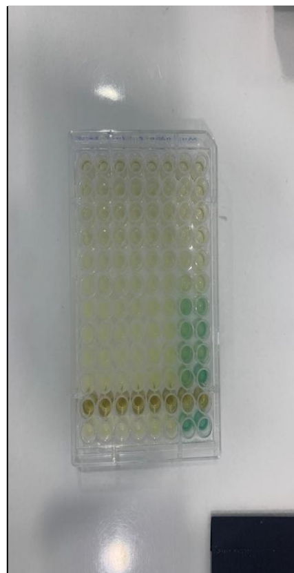
Figure .2: Representative 96-well microtiter plate illustrating the determination of Minimum Inhibitory Concentration (MIC) for tested extracts against selected microbial strains. Serial dilutions were performed across wells, with observable turbidity or colorimetric changes indicating bacterial growth, and clear wells representing inhibitory concentrations.
