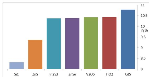
Fig. 5, d: The conversion efficiency of all cells after the addition of the buffer layer.
