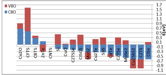
Fig. 4, c: Offsets of conduction and valance band values after adding the back reflection layer
