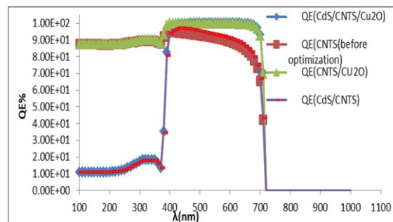
Fig. 9: Quantum efficiency as a function of the wavelength of the best studied cells.
