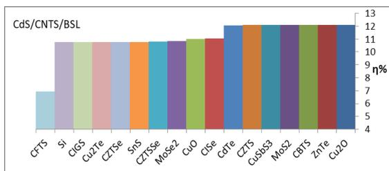
**Fig. 6, b: Results of solar cells after adding all the BSL with CdS layer.**
