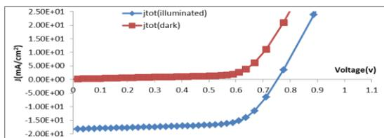
**Fig. 3: Dark and illuminated (J-V) of photovoltaic cell.**
