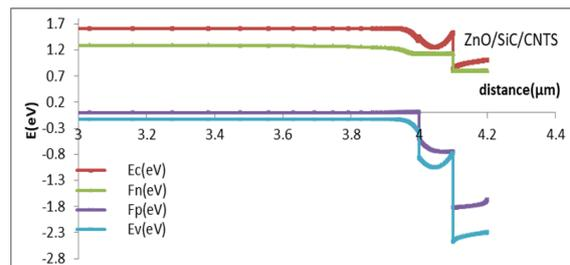
Fig. 5, c: Energy band diagram of SiC layer.
