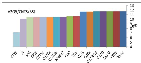
**Fig. 6, d: Results of solar cells after adding all the BSL with  $V_2O_5$  layer.**
