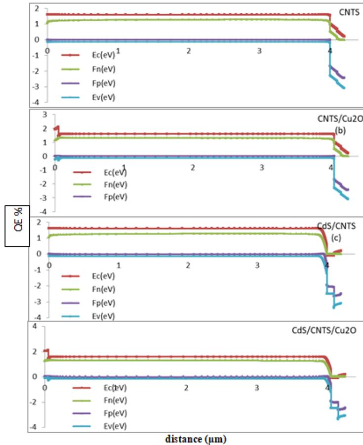
Fig. 8: Energy diagram (a) Cell before optimization (b) The cell after adding the reflection layer (c) The cell after adding an buffer layer (d) The cell after adding the reflection and buffer layer.
