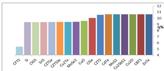
**Fig. 4, a:** Shows the conversion efficiency of cell different reflection materials.
