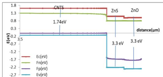
**Fig. 2: Energy band diagram.**
