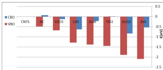
Fig. 5,a: Offsets conduction and valance band values after adding the buffer layer.
