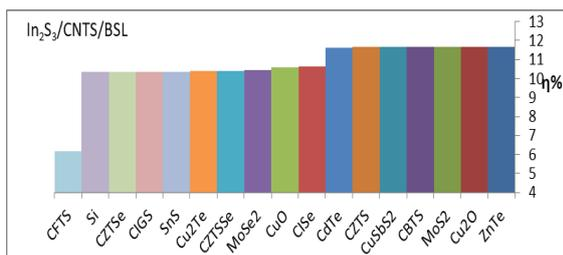
**Fig. 6, e: Results of solar cells after adding all the BSL with  $In_2S_3$  layer.**
