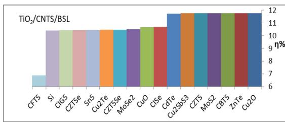
**Fig. 6, c: Results of solar cells after adding all the BSL with  $TiO_2$  layer.**
