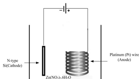
**Fig. 1:** Schematic diagram of a conventional ECD cell.
