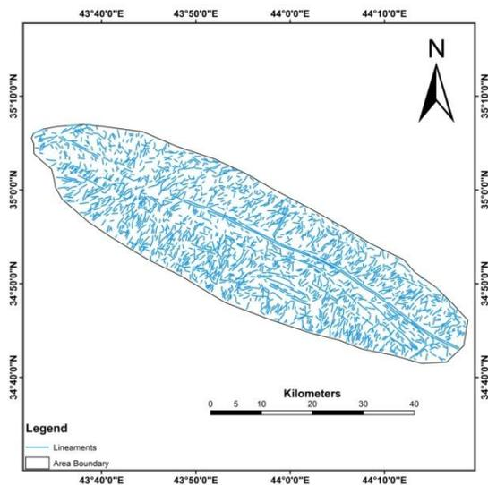
**Fig. 6: Automatically extracted lineaments in the study area.**
