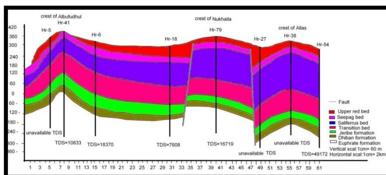
Fig. 15: Longitudinal geological cross section along Hemrin oilfield
