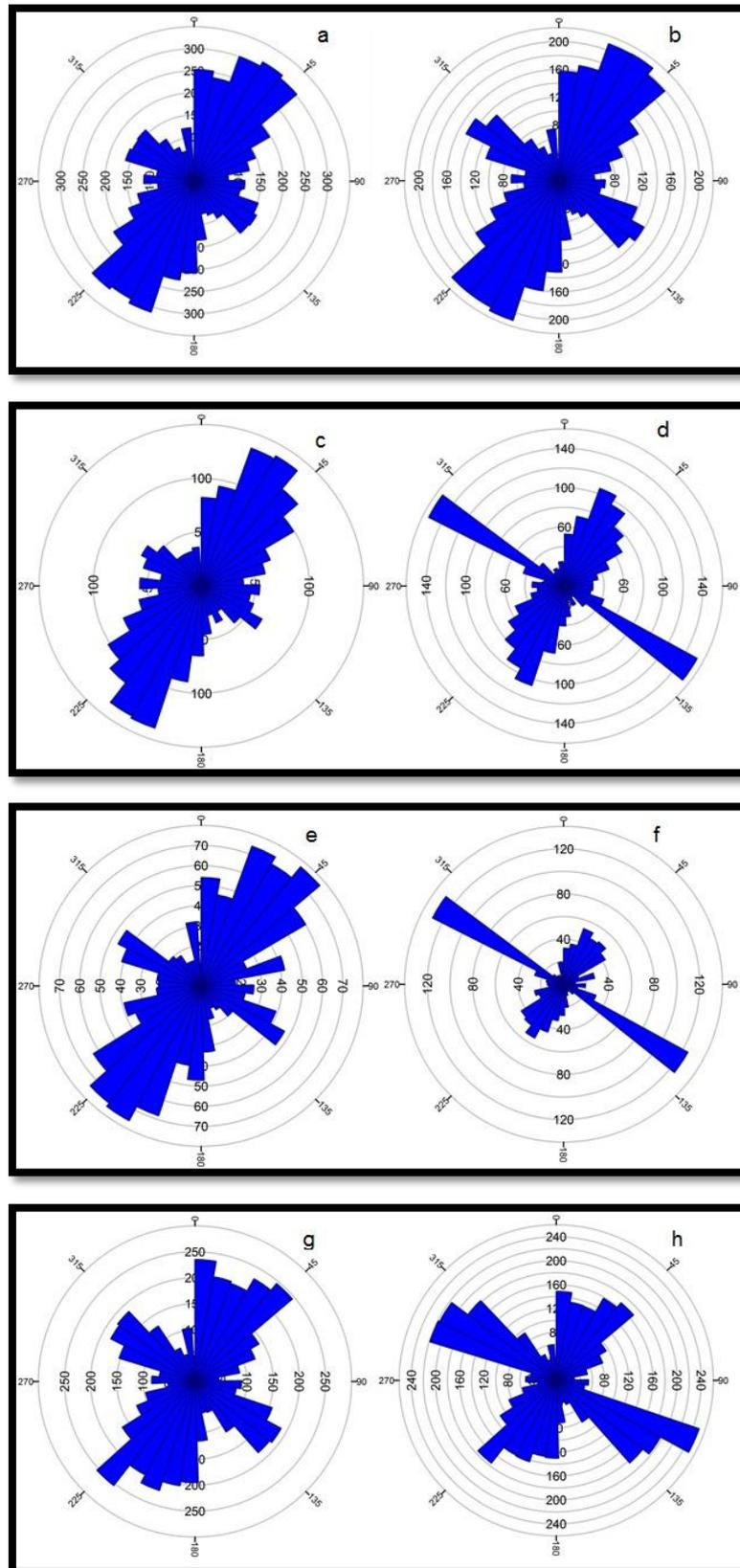
**Fig. 9:** Shows rose diagram analyses for the detected lineaments in Hemrin structure (a) Lineaments frequency of three domes (b) Lineaments length analysis results of the three domes (c) Lineaments frequency of Albufudhul dome (d) Lineaments length analysis results of Albufudhul dome (e) Lineaments frequency of Nukhaila dome (f) Lineaments length of Nukhaila dome (g) f Lineaments requency of Allas dome (h) Lineaments length analysis results of Allas dome.
