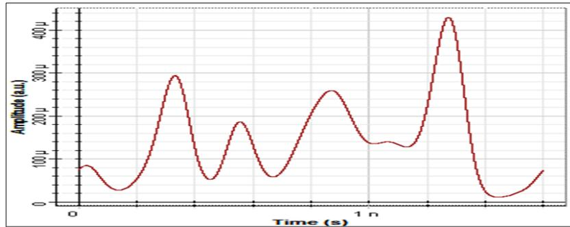
Figure 14: Output Signal\_3(193.3THz), after PIN from oscilloscope visualizer.
