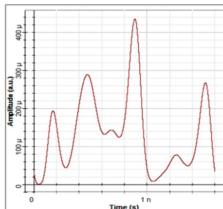
Figure 13: Output Signal\_2(193.2THz), after PIN from oscilloscope visualizer
