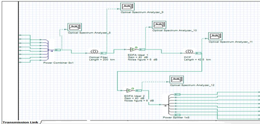
Figure 6: Clarifies the optical transmission link subsystem
