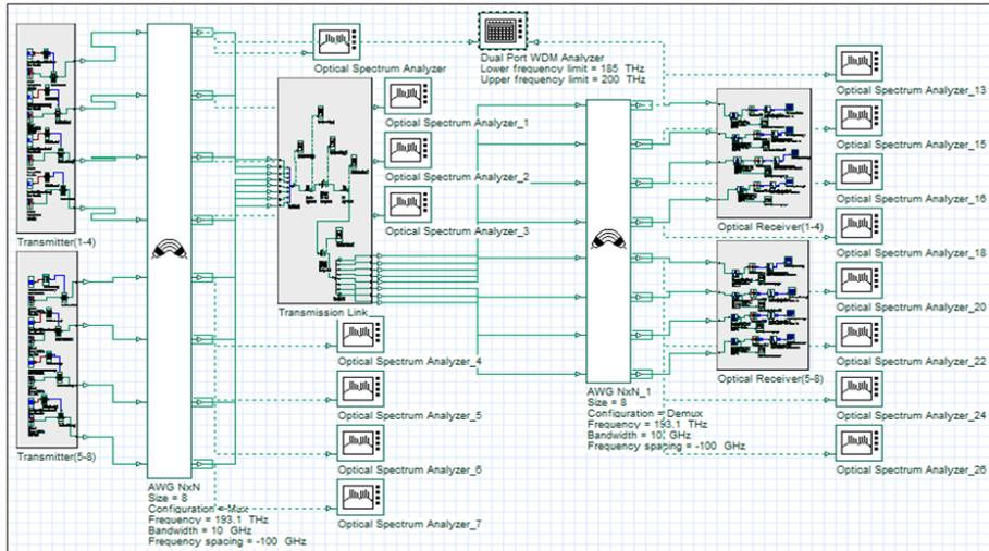
Figure 3: The Block Diagram of AWG architecture.
