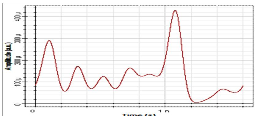
Figure 19: Output channel\_8 (1546.92nm) output after PIN from the oscilloscope visualizer
