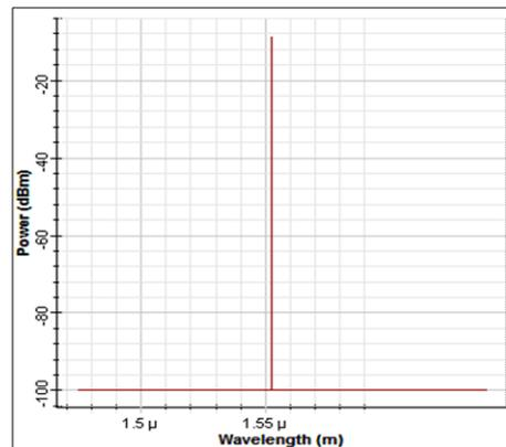
Figure 12: The output channel\_1(1552.52nm) after optical filter
