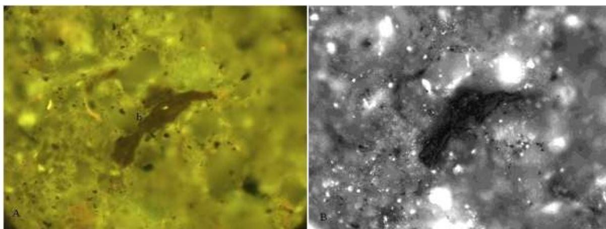
**Plate 4. (A): Brown fluorescing unstructured organic matter (bituminite) (b). Incident light fluorescence mode. B: Same section as A but in an incident light. Akkas-3 well, 1240 m. Oil immersion, X400**
