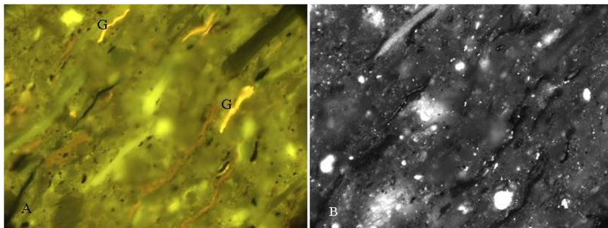
**Plate (1) A: Brightly fluorescing lamina consisting of alginite particles (G). Incident light fluorescence mode. B: Same section as A but in an incident light. Akkas-1 well, 1382 m. Oil immersion, X400**
