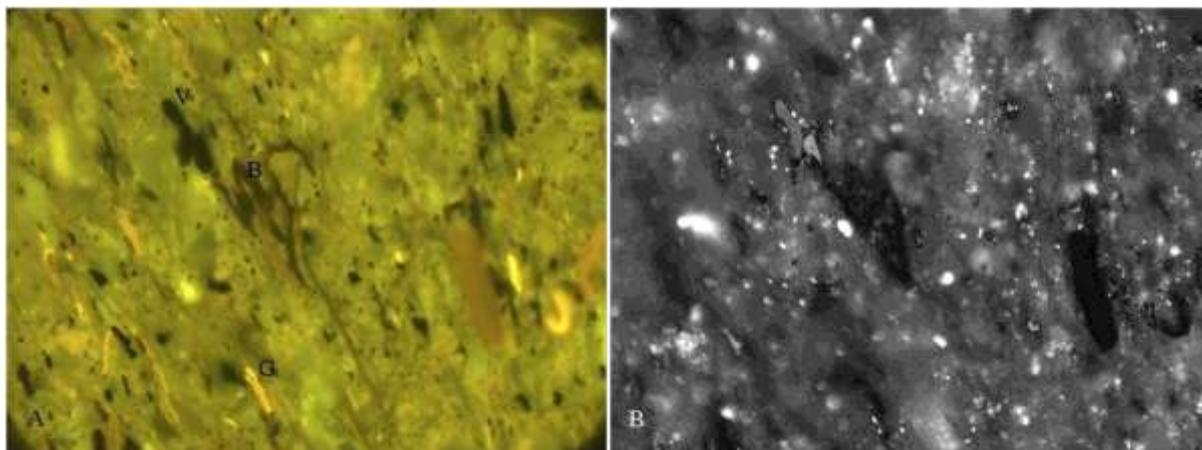
**Plate 3: (A): Brown fluorescing bituminite (B) with yellow fluorescing alginite (G) and vitrinite (V). Incident light fluorescence mode. B: Same section as A but in an incident light. Akkas-3 well, 1243 m. Oil immersion, X400**
