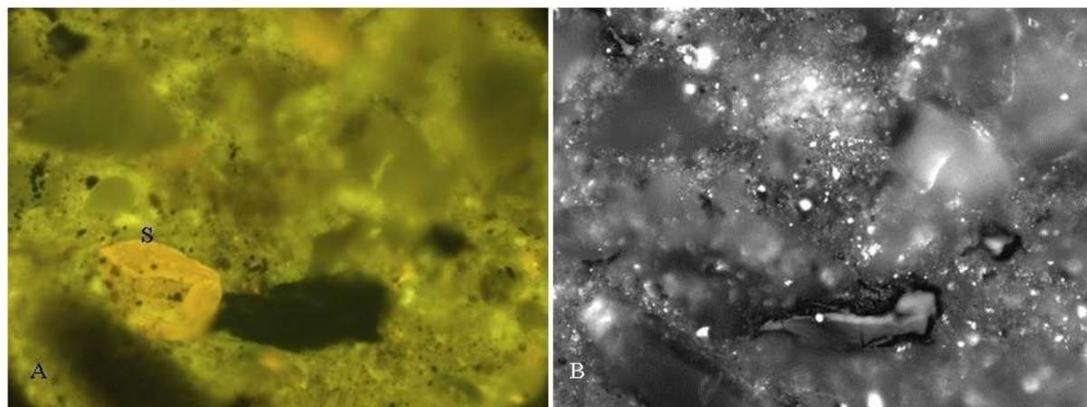
**Plate 5. (A): Strongly yellow fluorescent sporinite (S). Incident light fluorescence mode. B: Same section as A but in an incident light. Akkas-1 well, 1320 m. Oil immersion, X400**
