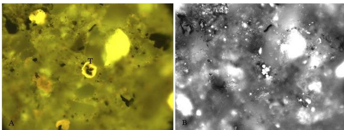
**Plate 2: (A): Strongly yellow fluorescing *Tasmanite* alginite (T). Incident light fluorescence mode. B: Same section as A but in an incident light. Akkas-3 well, 1233 m. Oil immersion , X400**
